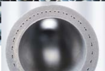
Hydraulic expansion of the tube pair Cross section of a tube pair after expansion
